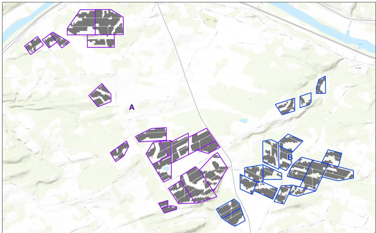
Figure 1: Mill Point Solar project PV panel layout (gray) with sub-arrays for GlareGauge assessment (purple and blue outlines)
